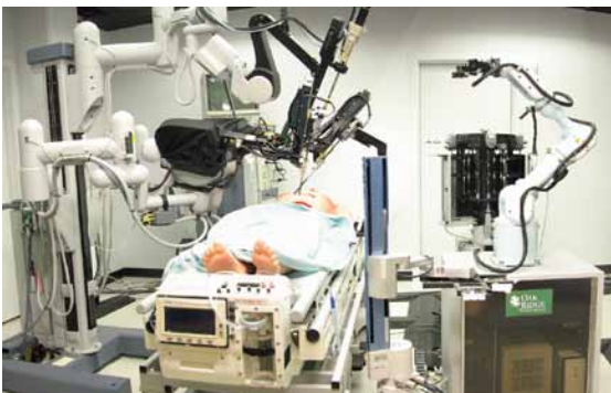
The Trauma Pod system, prototyped at SRI International, enables remote diagnosis and treatment of soldiers wounded in combat.
