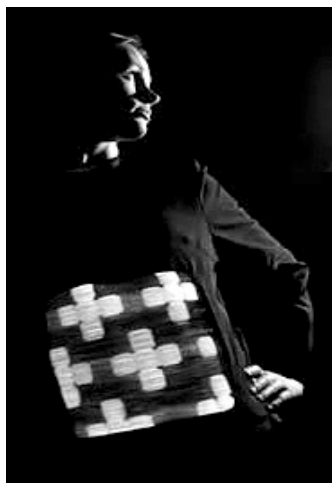
Figure 22 France Telecom's Optical Fiber Display Is a Fabric
