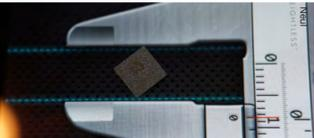
WHITE-SPACE RADIOS The UK's Weightless Special Interest Group has developed a chip that uses unlicensed low-frequency TV airwaves for wireless machine-to-machine communications.
